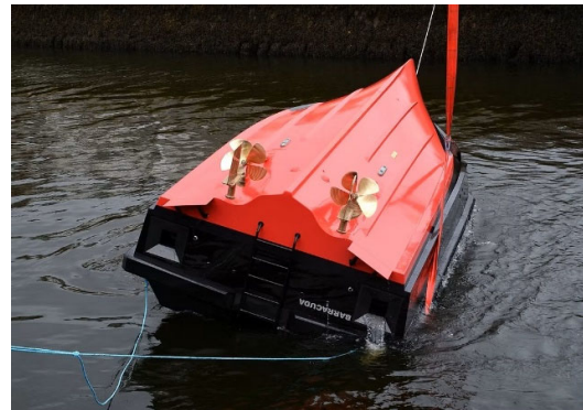
Barracuda – self-righting trials (Safehaven Marine)
